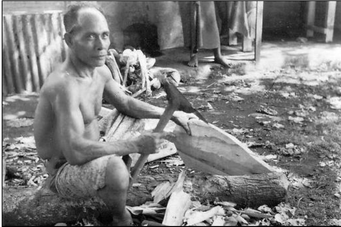
Falili, the lead carver (tufuga fau va'a) using that adze to carve the paddle (foe) of the paopao.
